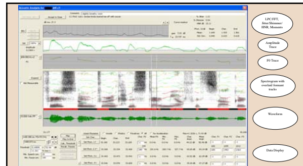
Figure 2 is a display of the analysis window for all acoustic measurements. Moving from the top of the window are: the comment box, the utterance gloss from the transcript, jitter/shimmer/HNR data, the LPC/FFT window, moment data display, the amplitude trace window, the F0 trace window, the spectrogram window, the waveform window, and the data window including data display for all measured data. For this figure the jitter/shimmer/HNR data is displayed for the segmented vowel (phoneme #16 in this utterance: /a/)
